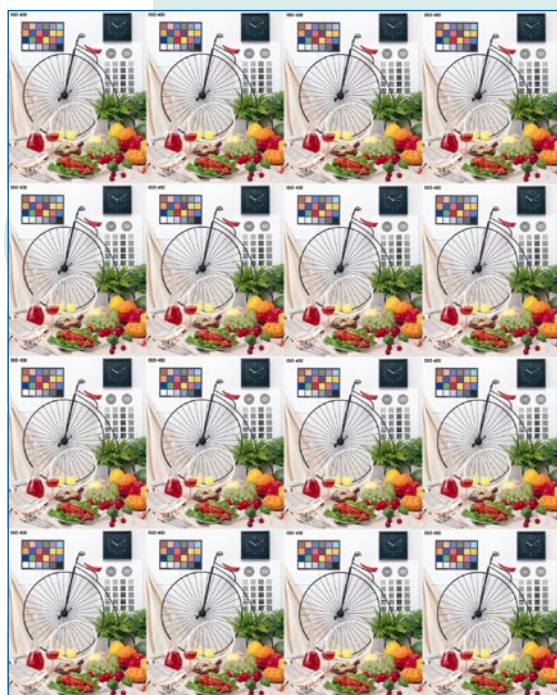
Test image used in BLI test comprised of 4 x 4 tiling of the ISO/JIS SCID No.5 Test Pattern
